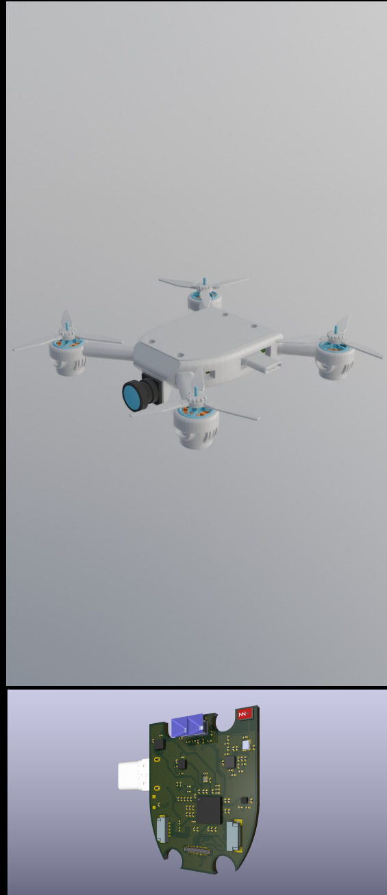
Figure 4: Top: Complete assembly of the drone. Bottom: Main controller board, top component layer.
